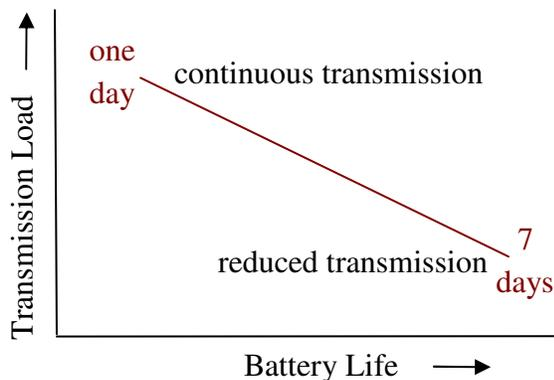
**Figure 3. Body Sensor Unit Improvement Potential.**
